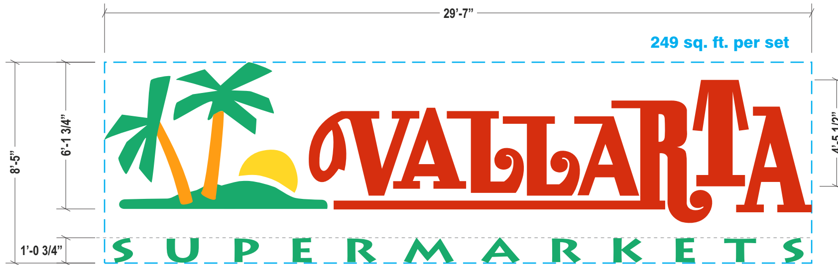
C SIGN-C: LED ILLUMINATED PAN CHANNEL LETTERS & LOGO Scale: 1/4" = 1'-0"
