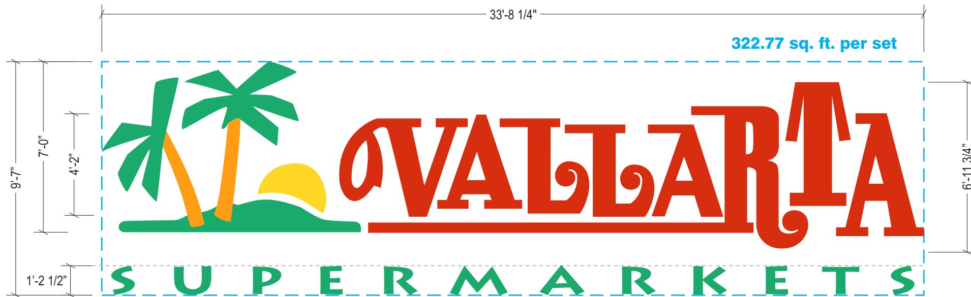
A SIGN-A: LED ILLUMINATED PAN CHANNEL LETTERS & LOGO Scale: 1/4" = 1'-0"
