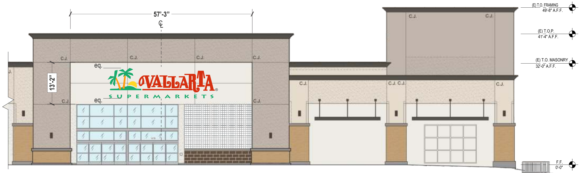
PARTIAL FRONT ELEVATION - WEST Scale: 1/16" = 1'-0"
