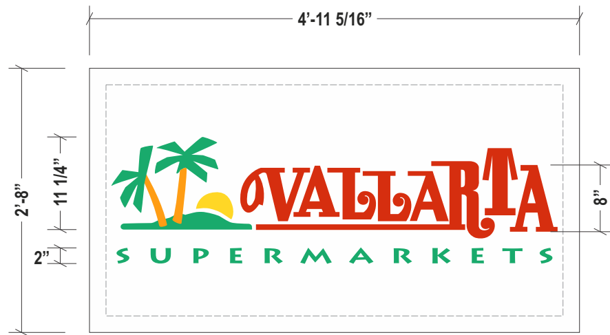
SIGN-M1 & M2: FACE ELEVATION Scale: 3/4" = 1'-0"
